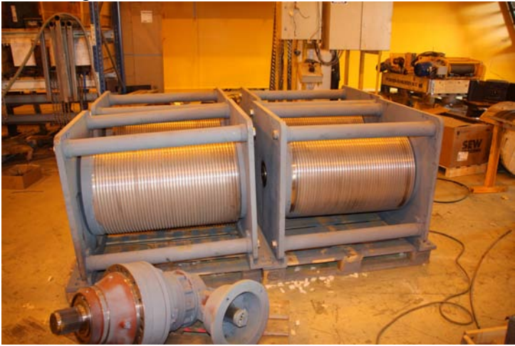
4 hoisting drums for a BOP offshore crane. The crane shall be on site 1.6.09
